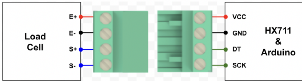
Figure 8: Data Processing - Connection with Terminal Blocks
